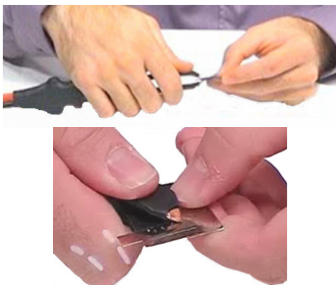
Figure 3: The tweezer hand piece (THP) being used to weld thin sheet metal.
