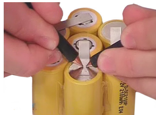
Figure 1: A cordless drill battery pack being welded using the dual probe hand piece (DPHP) welding attachment.
