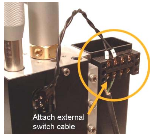
Figure 15: The ESHC external switch hookup cable attaches to the SEK500 as shown.
