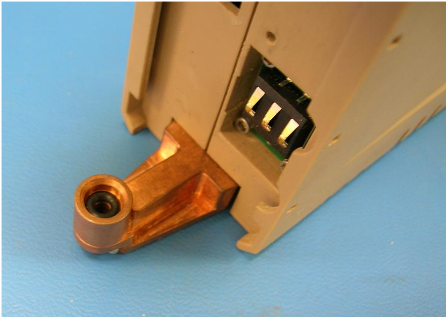
Figure 2: Cartridge installation (continued): The cartridge nozzle will mate with the nozzle acceptor shown in the above picture.
