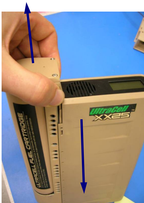
Figure 3: Cartridge removal: Push cartridge eject tabs in to unlock cartridge and pull cartridge out of system
