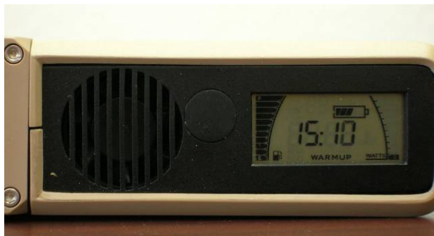
Figure 5: LCD display during system startup. Press the LCD backlight button quickly and repeatedly to adjust LCD contrast.
