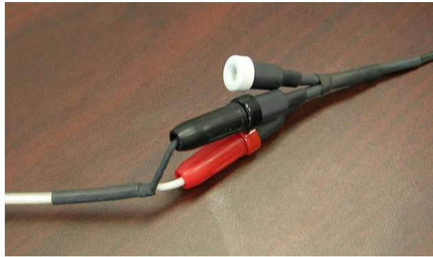
Figure 4: Connect XX25 to your Application using supplied tether. Red banana plug is Power, Black is Ground.
