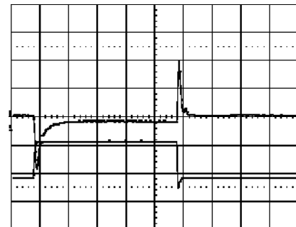
Output voltage response to load current step- change (15-30-15 A) at: T_{ref} = +25^{\circ}\text{C} , V_i = 53\text{ V} . Trace: output voltage (100mV/div.). Time scale: (0.1 ms/div.).
