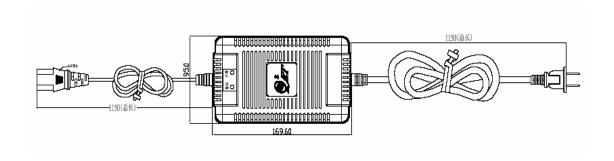
Tolerance of outline dimension is  $\pm 0.5$ mm, others are  $\pm 0.2$ mm in the diagram;
