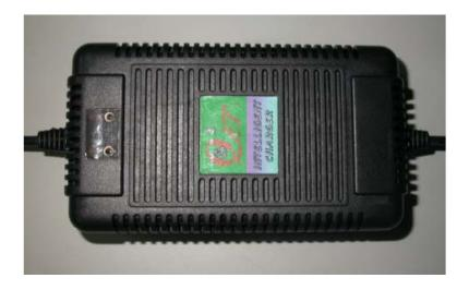
Power supply QQE048-5CH71 is cooled No fan, can work normally under 14.5Vdc/ 4A, featuring output current limiting protection, short circuit protection, It's designation strictly follows EMC requirements, meets requirements of household electrical equipment standards and gets CE certification.
