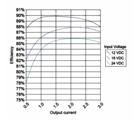
Figure 1 Typical efficiency curves PowerStream Technology PST-DCZ0930 3/12/08
