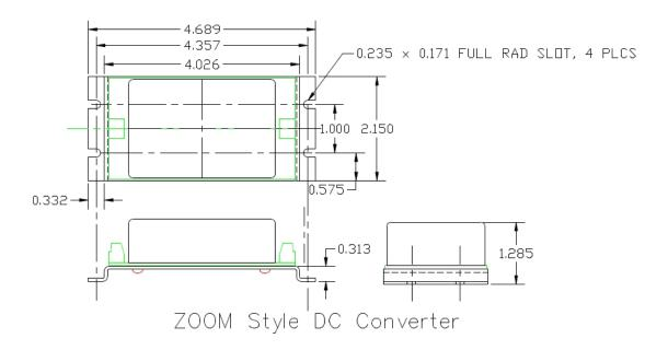
Figure 2. Dimensioned drawing.
