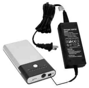
3. MP3450I will be charged fully in 4 hours or so, while the charge LED indicator turns green. (If you want to know the capacity status, please press Capacity Display Button, the LEDs will indicate the accurate capacity status. It indicated fully charged when all the LEDs are light.)
