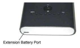
Press the button on the top cover of MP3460, and the LEDs will indicate the capacity status.
