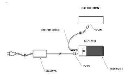
According to the way of the connection, the product can offer power to instrument and charge MP3450I at the same time. When the AC power is shut down, that's to say, the output voltage of AC power adapter is 20% lower than normal, the MP3450I will be exchange the battery power to the connected instrument. So it's same as the UPS function(uninterrupted power system).
